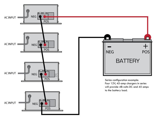
This illustration demonstrates a typical series configuration system. When the battery chargers are connected in series, the system delivers increased output voltage (output voltage x number of chargers) but no change in amperage.
