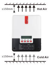
Figure 2-1 Installation and Heat Dissipation
