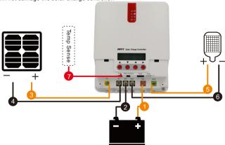
Figure 2-3 Wiring
