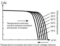
Figure 1-4 Solar Panel Output
