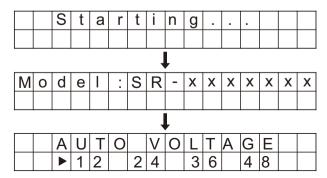
During start, the four indicators flash in flow. LCD starts after self-check. The model of the solar charge controller is displayed first, and then battery voltage level is displayed. Voltage level is displayed according to user-selected fixed voltage or voltage automatically identified.
