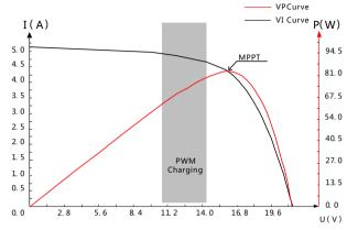
Figure 1-2 Solar Panel Output Characteristic Curve
