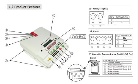
Figure 1-1 Solar Charge Controller Appearance and Interface
