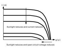
Figure 1-3 Solar Panel Output Characteristic and Lighting Relation
