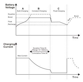
Figure 1-4 Battery Charging Stage
