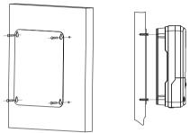
Figure 2-2 Fix the solar charge controller
